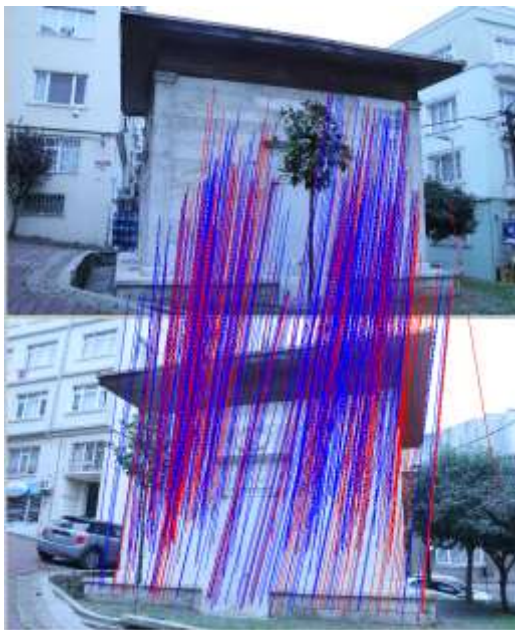
Figure 7. The matching points in two photos
