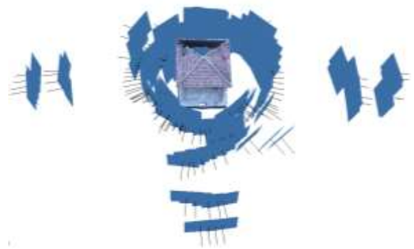
Figure 5. Automatically calculated camera positions
