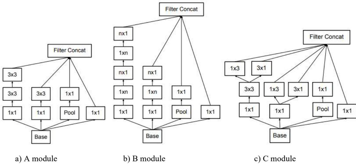
Figure 5. The modules used for Inception V2 network [13].
