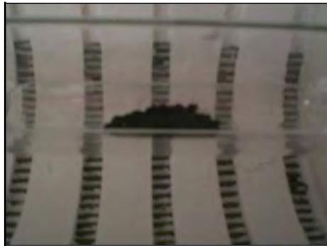
**Figure 2.** The photograph of synthesized CNTs in quartz boat
