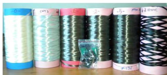
Figure 8. PAN /CNT nanocomposite fibers: (Fiber0) PAN, (Fiber-CNT3) fiber produced by former studies (0.02% acrylic acid PF-CNT + SDBS), (Fiber1) 0.2% PF-CNT + SDS, (Fiber 2) 0.2% PF-CNT + Triton X100, (Fiber 5) 0.2% PF-CNT, (Fiber 4) 1.0% PF-CNT + SDS and (Fiber3) (front) 0.4% PF-CNT + SDS
