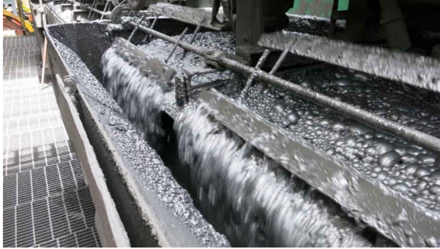
Figure3. Accumulating mineral installed bubbles at an industrial zinc ore dressing application (Northern miner, 06.05.2022)
