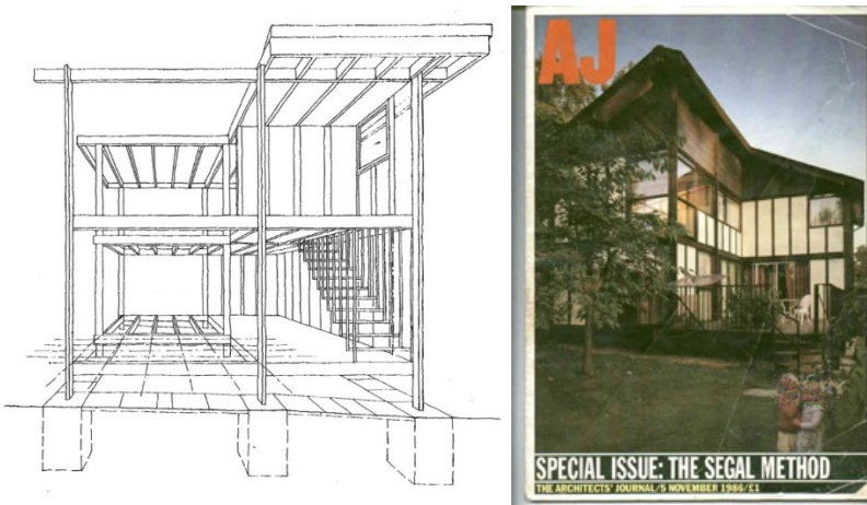
Figure 6. Principles of Segal Method (left) and its application (right) (“Special Issue: The Segal Method,” 1986)
