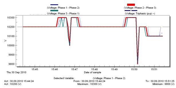
Figure 4. Voltage change of the motor during start up.
