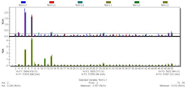
Figure 7. Indivudial harmonic spectrum of voltage and current at power plant.
