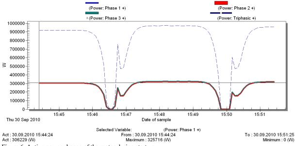
Figure 6. Avtive power change of the motor during start up
