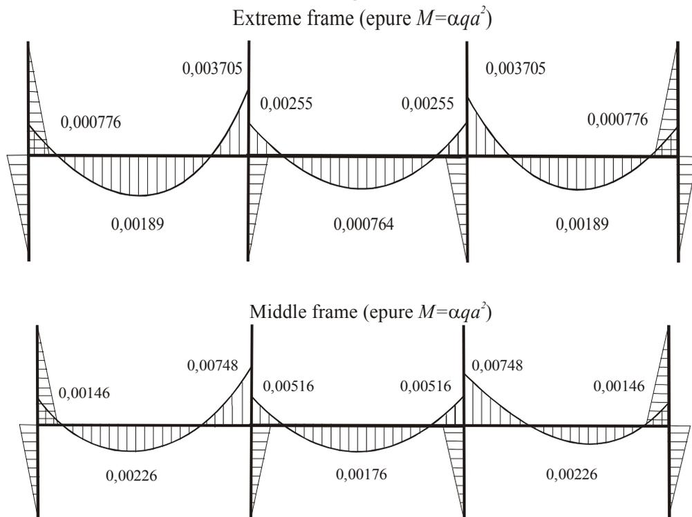
Figure 2. Epure of bending moments of beam floor slabs. ( Continue )
