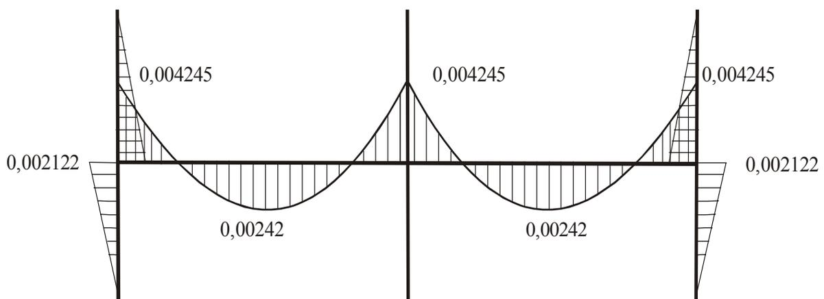
**Figure 2.** Epure of bending moments of beam floor slabs
