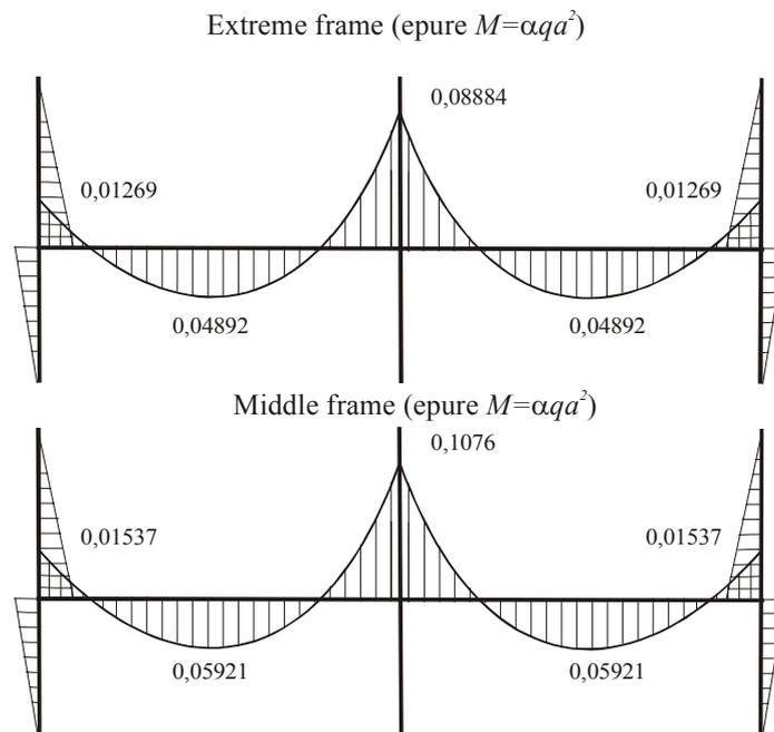
Figure 3. Epure of bending moments of beamless (flush) floor slabs.
