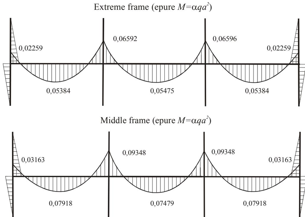
**Figure 3.** Epure of bending moments of beamless (flush) floor slabs. ( Continue )
