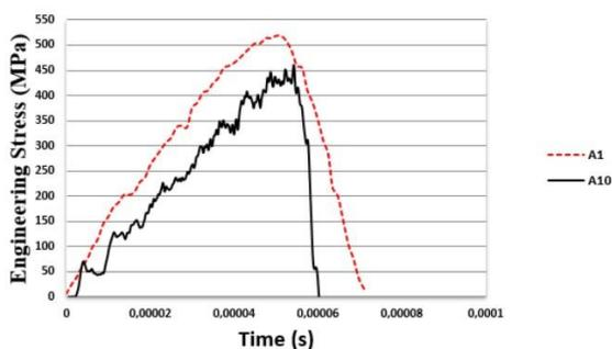
Figure 18. Comparison of stress and time with varying fibre orientation under out of-plane loading conditions (Fibre Orientation:90<sup>0</sup>)
