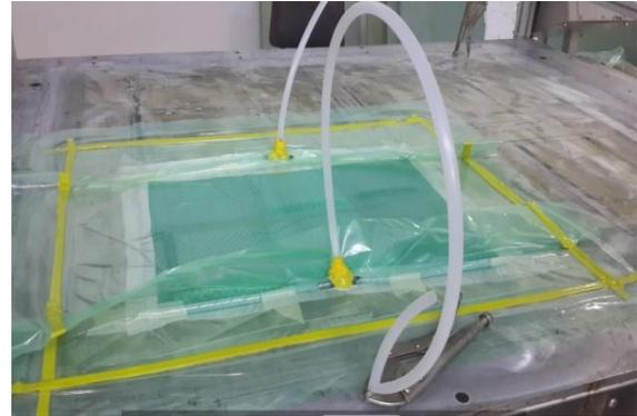
Figure 2. Production of composite layers
