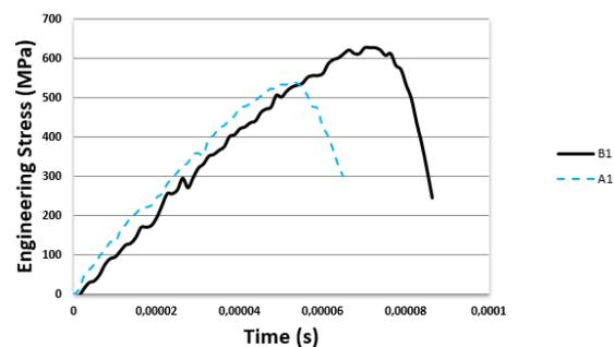
Figure 11. The stress-time curves of the specimen under out-of-plane loading
