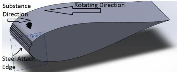
Figure 8. Illustration of impact processing to blade
