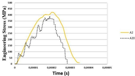
Figure 17. Comparison of stress and time with varying fibre orientation under in-plane loading conditions (Fibre Orientation:90<sup>0</sup>)
