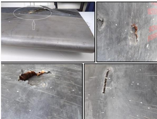
Figure 9. Damaged main rotor blade: Turkish Airforce Blade Repair Center
