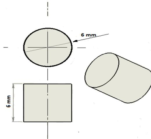
Figure 7. Geometry of a hard specimen prepared for SHPB
