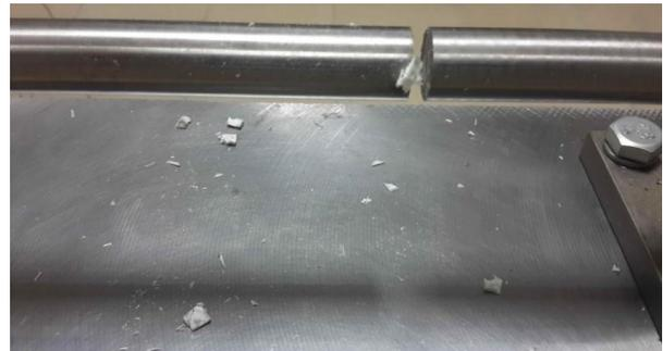
Figure 15. Disruption of the specimen under in-lane loading
