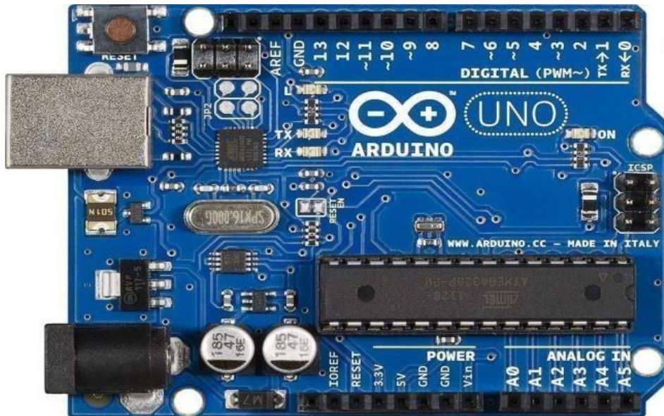
Figure 4 is the Arduino Uno installed in the project as the head, main controller.
