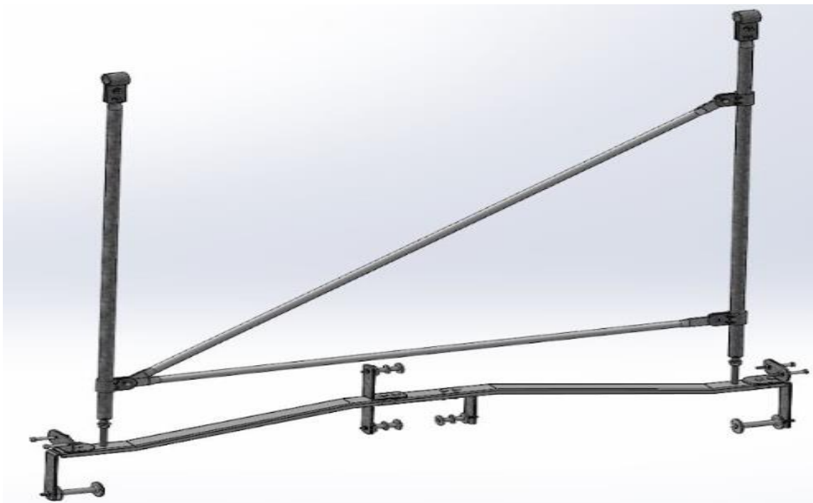
Figure 5. Solidworks design of irrigation system installation hanger set
