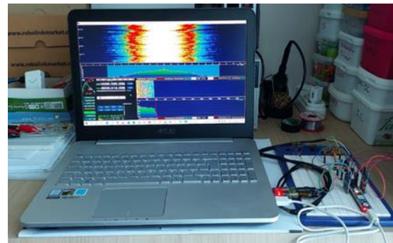
Fig. 4 Photo of the FMTX system in operation
