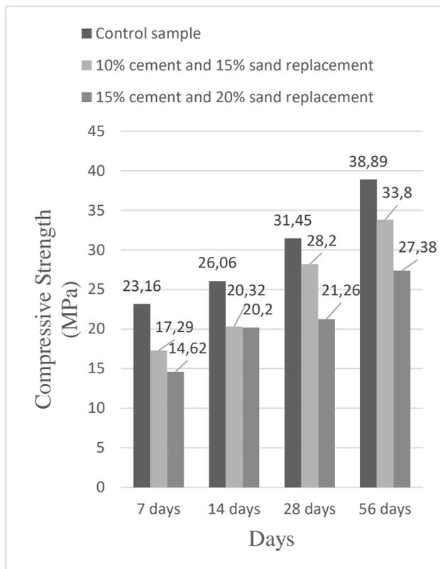
Figure 7: Compressive strength of comparison
