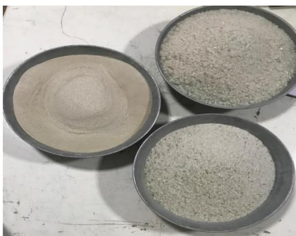
Figure 2: Sieved glass powder for cement and sand
