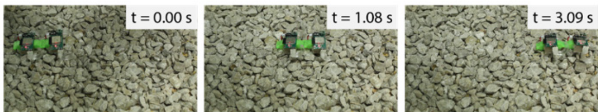
Figure 12. REMIRO with two modules moving on a surface covered with gravel.
