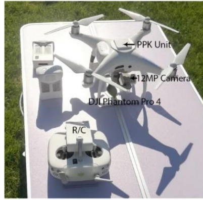
Figure 5 : The modified PPK based UAV platform used to acquire photogrammetric aerial-images used in the Experiments.
