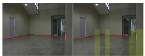
Fig. 9. Extracted corridor lines and certain horizontal gaps between the lines (left) and Treatment of Horizontal Gaps (right)
