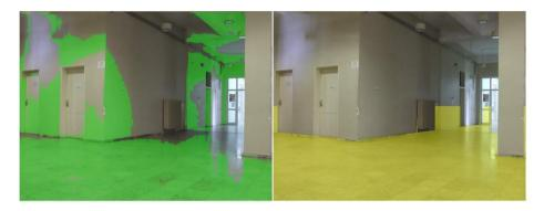
Fig.11. Flood fill results (left) and floor mask (right) on corridor image
