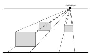
Fig. 6. One point perspective – image plate is parallel to Cartesian scene in two axes
