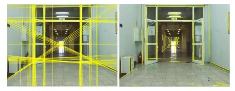
**Fig. 3.** Standard Hough Transformation (left) and Progressive Probabilistic Hough Transformation (right)
