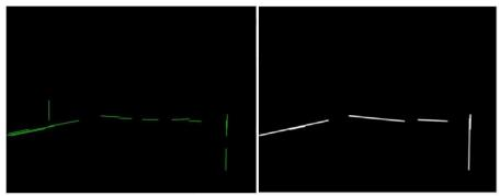
**Fig. 4.** PPHT results on the edge image are small line pieces (left), these pieces are merged through line clustering algorithm (right)
