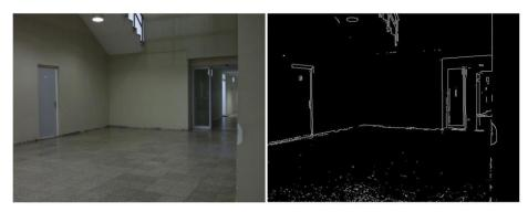
Fig. 2. Results of Canny Filter applied on the raw corridor image
