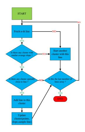
Fig. 5. Overview: The procedure of line clustering
