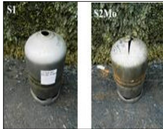
**Figure 5.** Cylinders subjected to bursting & volumetric expansion test
