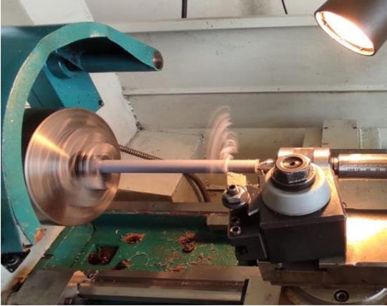
**Figure 2.** Turning process for 3D printed bolt shafts
