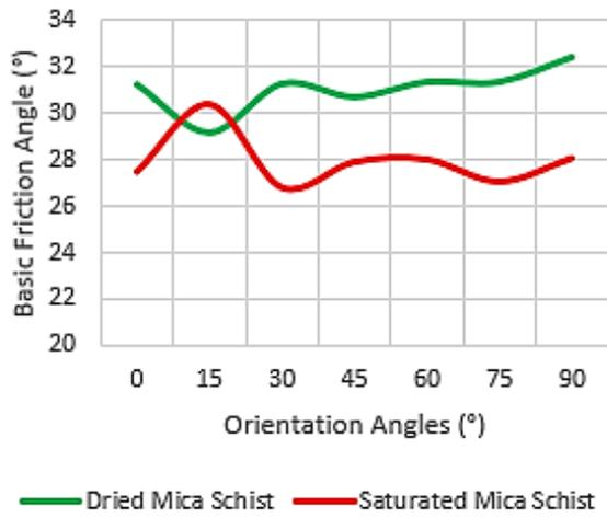
Figure 7. Basic friction angle values for mica schist.
