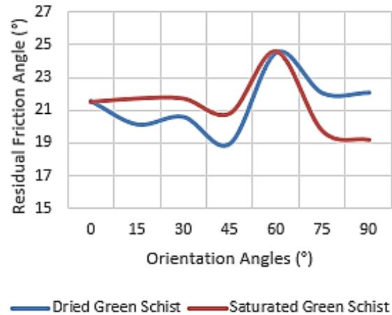
Figure 10. Residual friction angle values for green schist.
