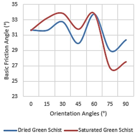
Figure 6. Basic friction angle values for green schist.
