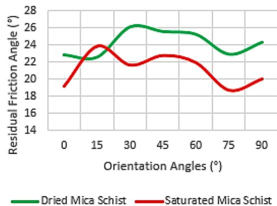
Figure 11. Residual friction angle values for mica schist.
