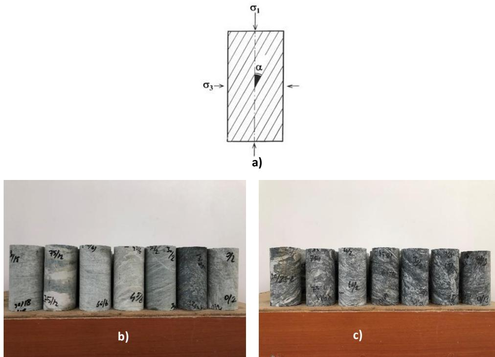
**Figure 2.** a) Orientation angle ( $\alpha$ ) b) green schist c) mica schist.
