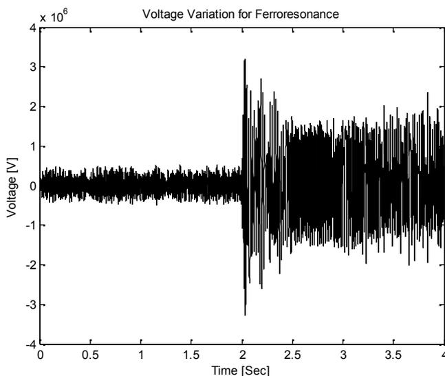
Figure 6. Voltage variation obtained from the extracted feature.
