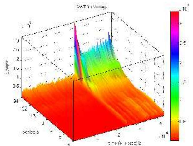
Figure 4. Three dimensional plot for the CWT of the voltage variation.
