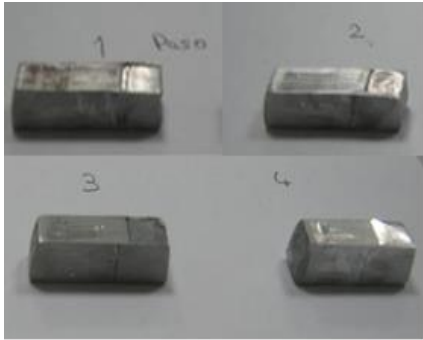
Figure 5. Examples of the ECAP specimens of several passes
