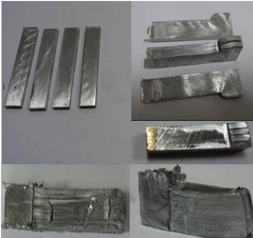
Figure 10. Strip ECAP'ing examples.
