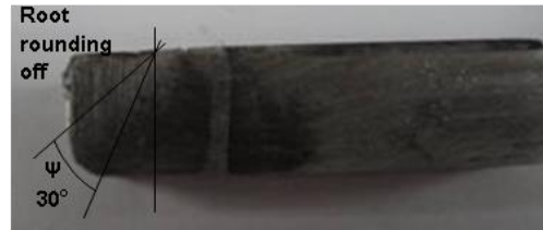
Figure 11. Occurrence of root rounding off in ECAP process
