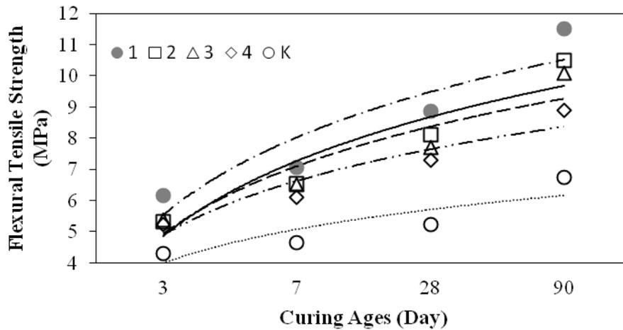
Figure 3. Flexural tensile strength test results of concrete series including single fibres
