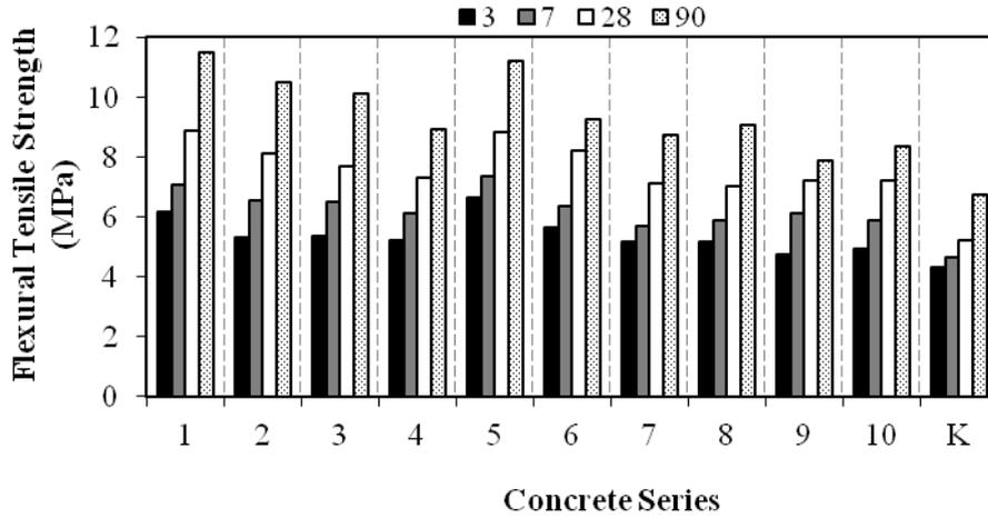
Figure 2. Flexural tensile strength test results of concrete series
