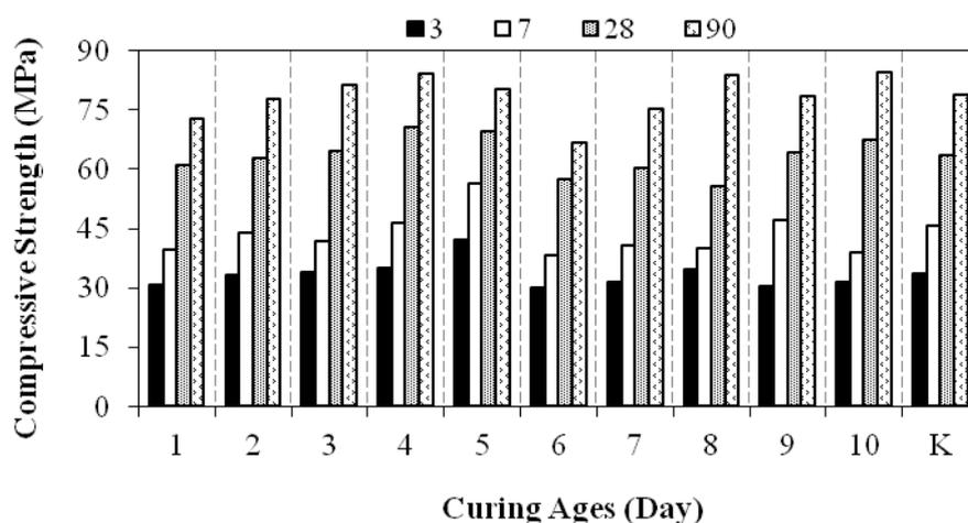
**Figure 1.** Compressive strength test results of concrete series
