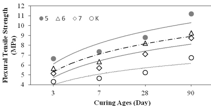
**Figure 4.** Flexural tensile strength test results of concrete series including 50% macro and 50% micro fibres
