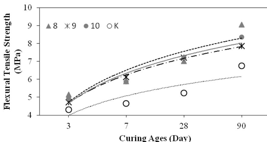
**Figure 5.** Flexural tensile strength test results of concrete series including 25% macro and 75% micro fibres
