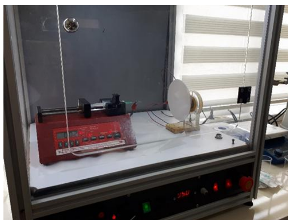
Figure 3. Electrospinning device used in experiments.
