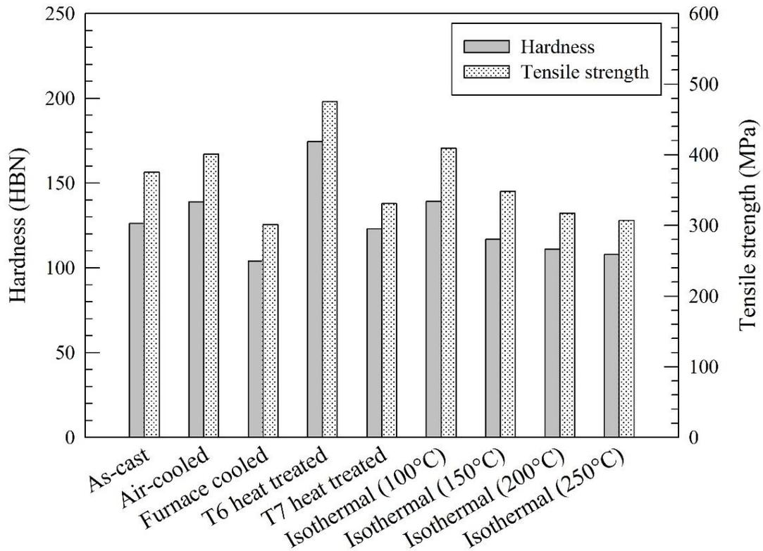
**Figure 1.** The bar chart showing the hardness and tensile strength of the alloy samples (Savaşkan et al., 2021; Savaşkan et al., 2022; Savaşkan et al., in press)
