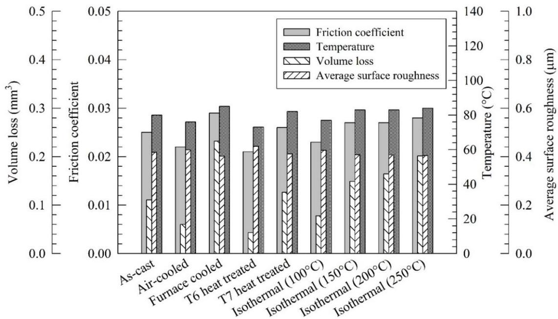
**Figure 2.** The friction coefficient, temperature, wear volume and average surface roughness values of the alloy samples (Savaşkan et al., 2021; Savaşkan et al., 2022; Savaşkan et al., in press)
