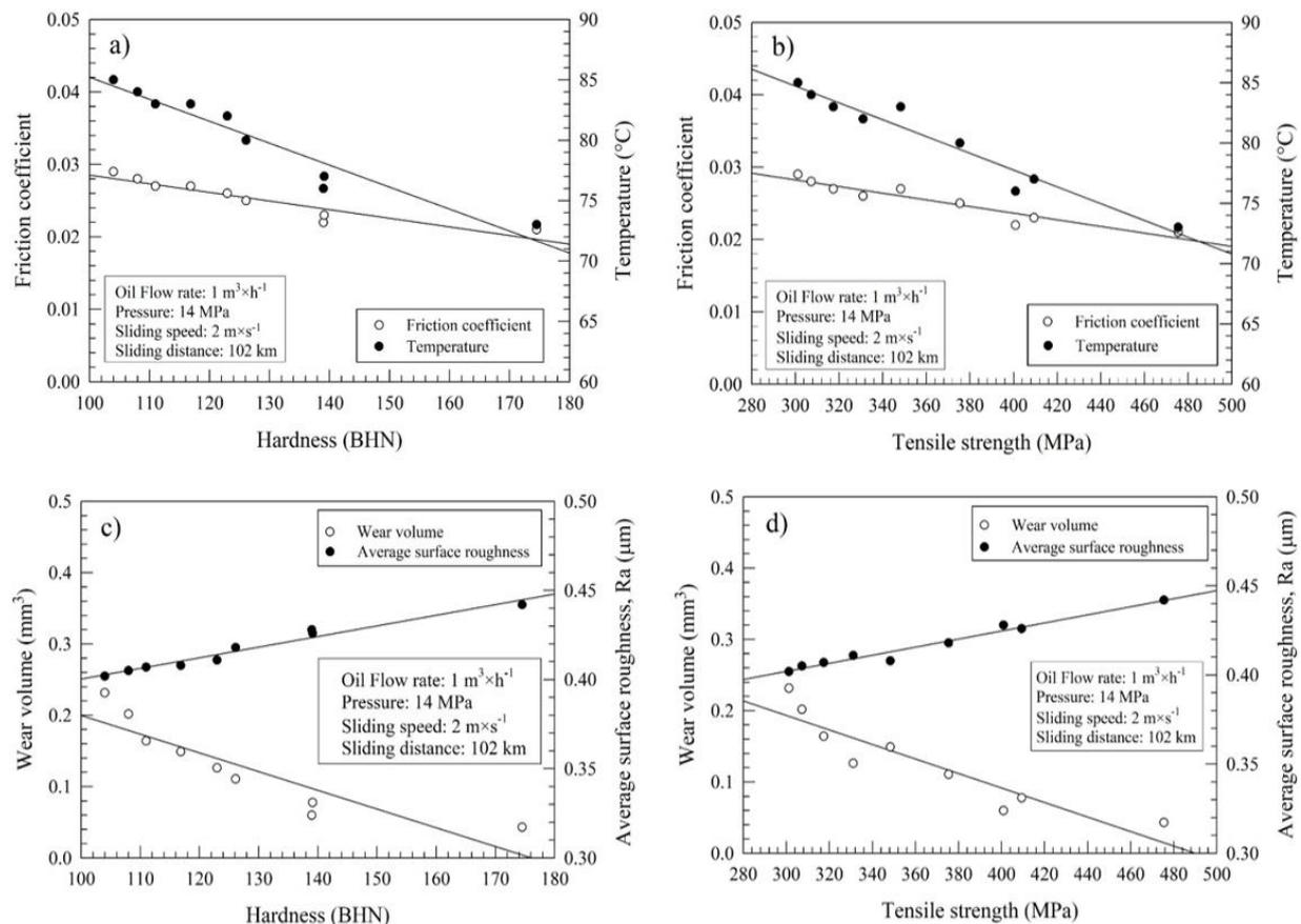
**Figure 3.** a) *FC* and *T* versus *H*, b) *FC* and *T* versus *UTS*, c) *WV* and *ASR* versus *H*, and d) *WV* and *ASR* versus *UTS* plots for Zn-40Al-2Cu-2Si alloy
