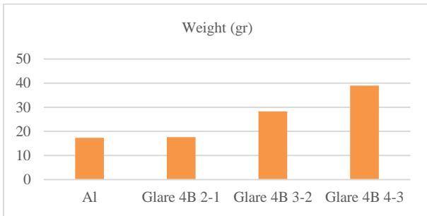
Figure 12. Weight of Glare 4B Grades and Al 2024-T3
