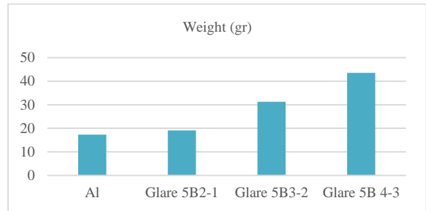
Figure 16. Weight of Glare 5B Grades and Al 2024-T3
