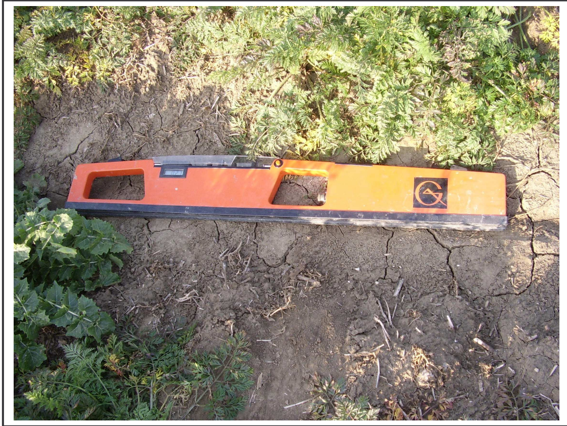
Figure 2. The EM38 placed horizontally to assess soil salinity over 0-1 m soil depth
