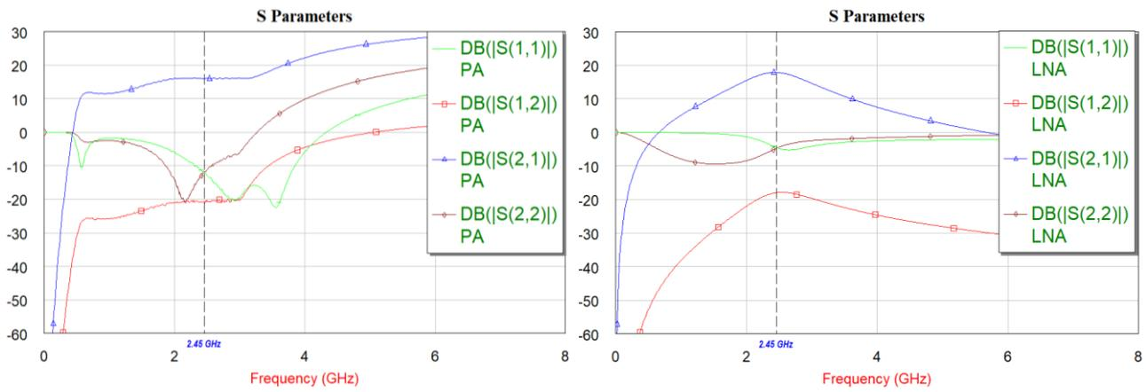
**Figure 3.** S Parameters of the PA & LNA circuits.
