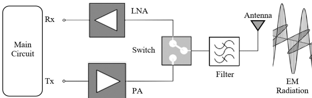
**Figure 1.** A basic front-end module.
