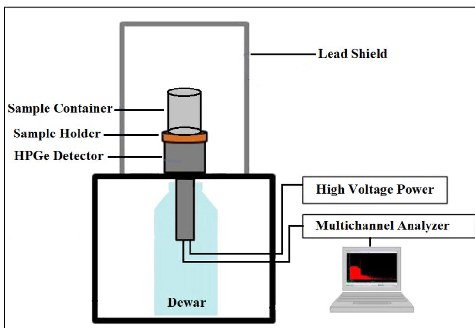
Figure 2. The experimental scheme of the gamma spectrometer system
