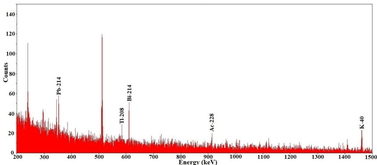
Figure 3. A typical spectrum image obtained from measuring samples at the detector
