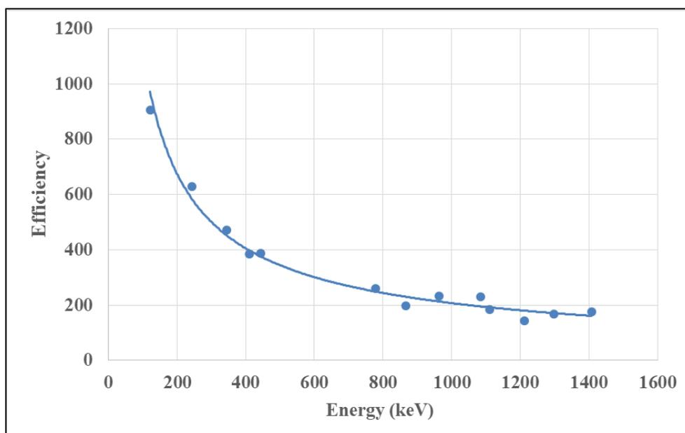
Figure 4. The efficiency graph obtained from Eu-152 standard source.
