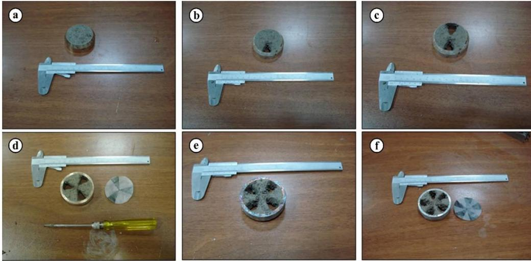
**Figure 4.** a) Intact soil sample (0% disturbance), b) 10% disturbed soil sample, c) 20% disturbed soil sample, d) 30% disturbed soil sample, e) 40% disturbed soil sample and f) 50% disturbed soil sample.
