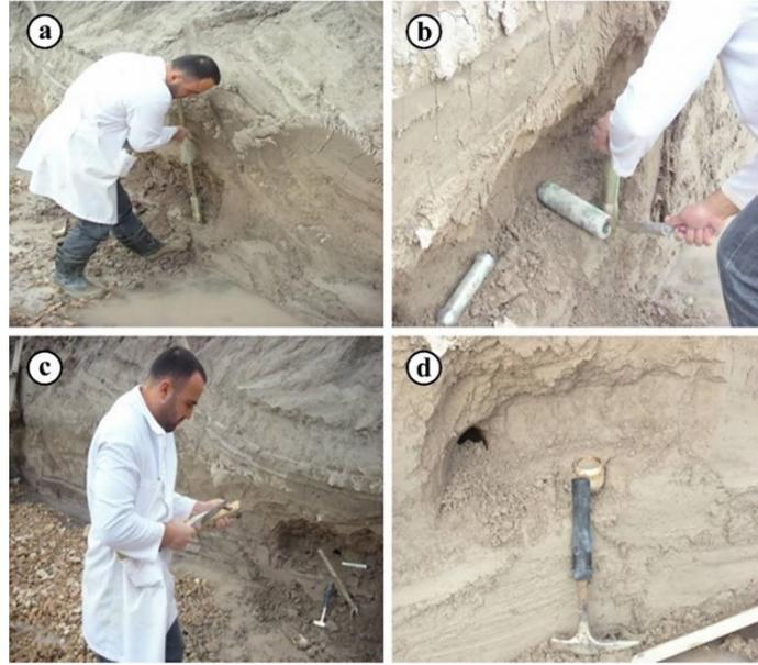
**Figure 2.** a) Tube sampling with sampling device, b) cleaning the outer side walls of the tube samples, c) waxing of the upper and lower parts of the tube samples, d) undisturbed soil sample image was taken into the consolidation ring.
