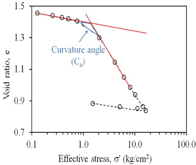
Figure 1. Approach to determine the curvature angle ( $C_a$ ).
