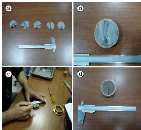
**Figure 3.** a) Percentage slices determined on transparent paper, b) marking the boundaries, c) marking the determined percentile on the soil sample and d) views of the slices to be emptied on the soil sample.
