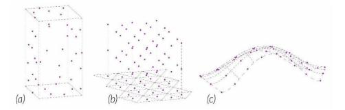
Figure 2. Point cloud generation approaches explored: a) random points in/on a bounding solid, b) 3D grid, and c) points on surface.
