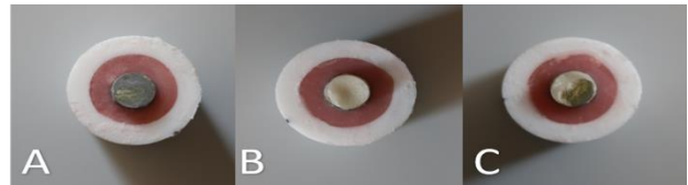
Figure 2: Failure modes; A: Adhesive, B: Cohesive, C: Mixed
