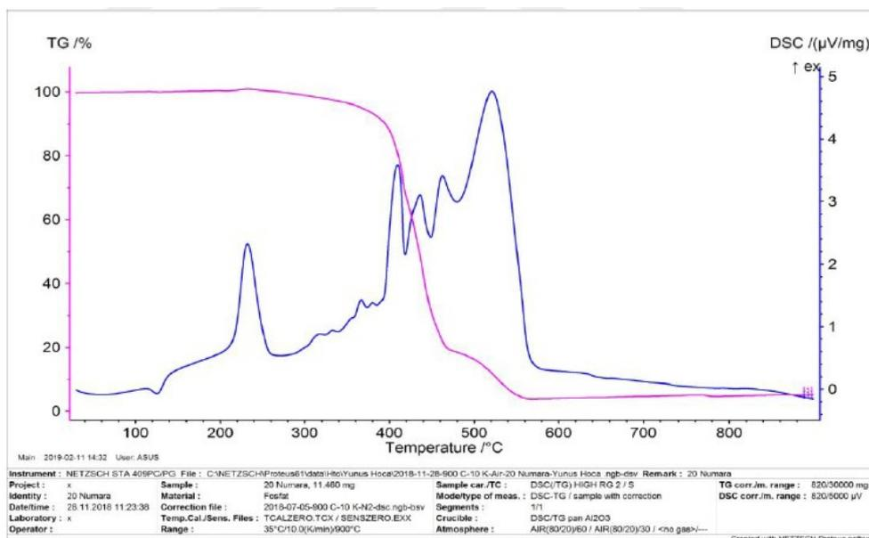
Figure 30. C-Tape sample (13) (PE+PET+Synthetic Rubber) thermal analysis chart.
