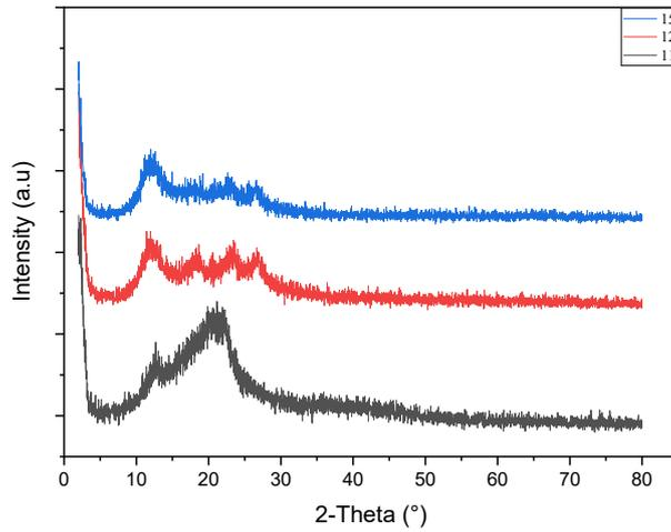
Figure 13. XRD graph of waste polymer in PET structure.
