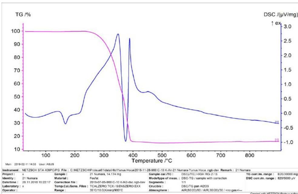
Figure 31. Flexible ear sample (14) (PP) thermal analysis chart.
