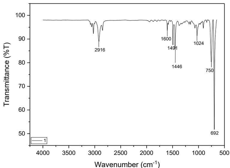
Figure 9. Facade ladding foam sample (PS) FTIR spectrum.
