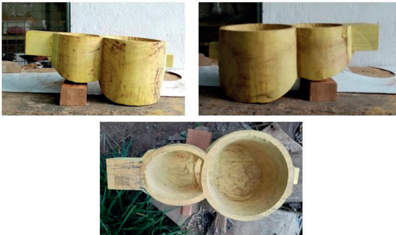
Figure 18. Right-side view of the physical resonator (upper left), left-side view of the physical resonator (upper right), and inside view of the physical resonator (bottom).
