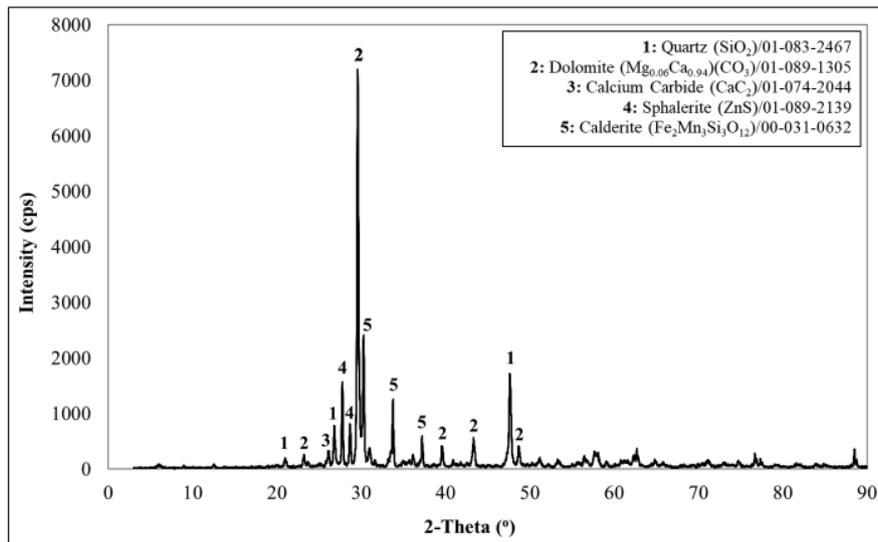
Figure 3. XRD diffraction figure of the sample
