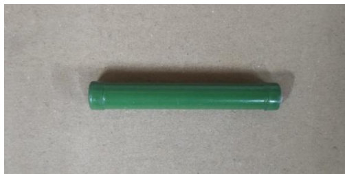
Figure 2. High voltage thick film resistor
