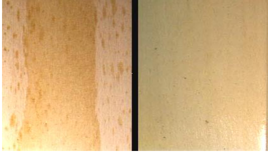
Figure 5. (Left) Natural image of Norway spruce, (Right) its image when densified with vibration [50].
