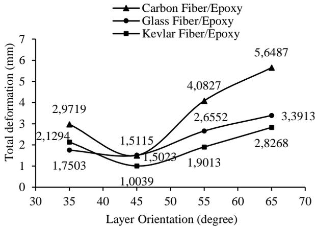
**Figure 8.** The graph of total deformations on pressure vessel at hydrostatic pressure of 11.25 bar
