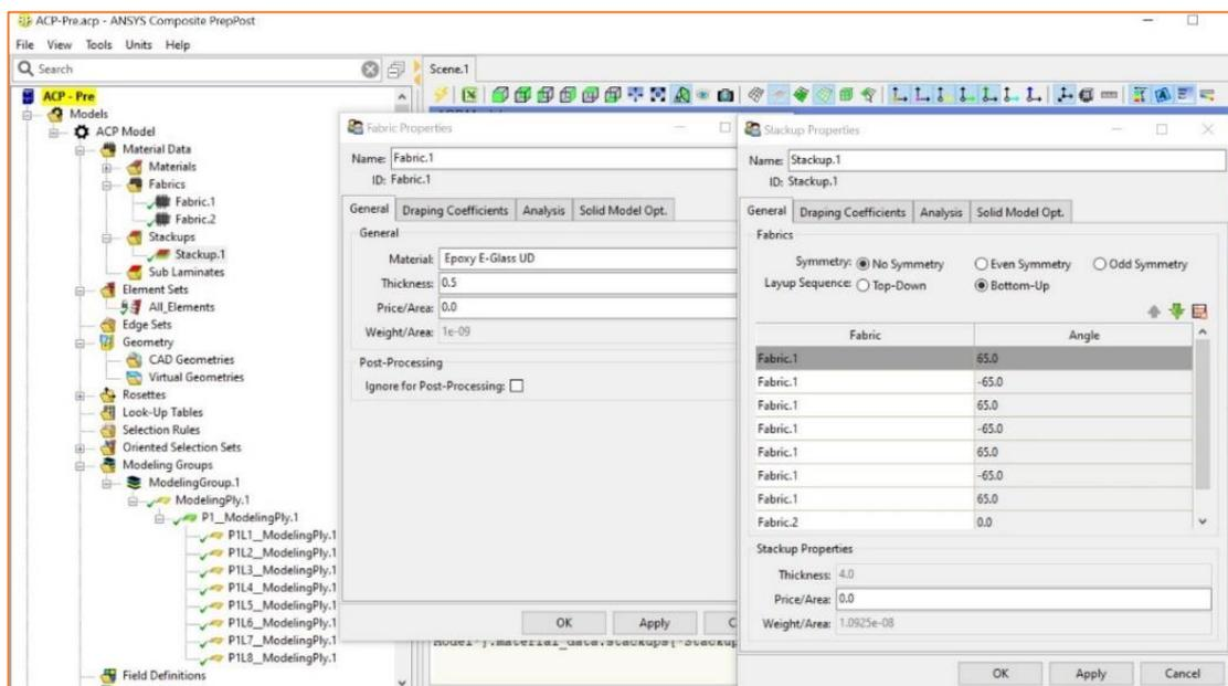
Figure 2. Display of material property, layer thickness, and orientation angles for epoxy E-glass
