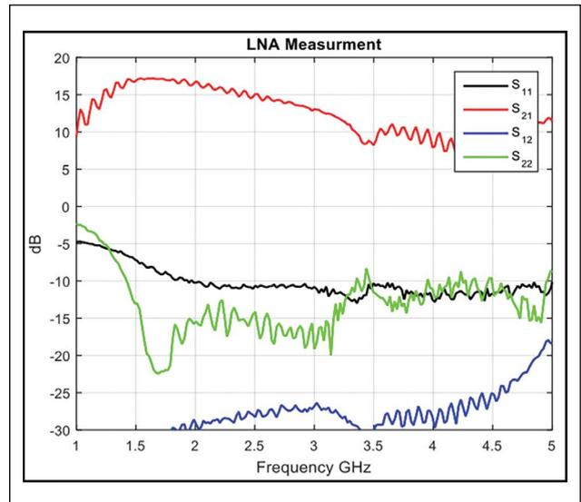
Figure 7. Measured S parameters of the LNA.
