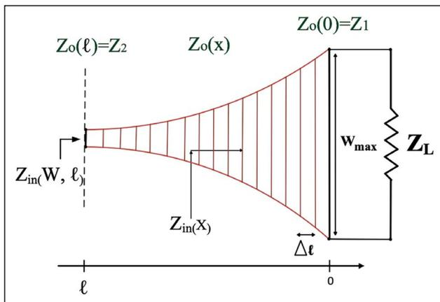
**Figure 1.** Schematic of an exponentially tapered microstrip line.
