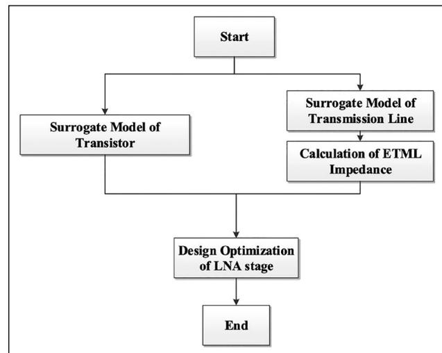
**Figure 2.** Flow chart of design optimization of the work.
