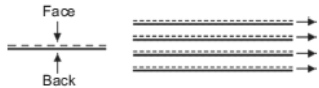
Figure 3. The placement of fabric plies performing "face up in a single direction" spreading mode [8].
