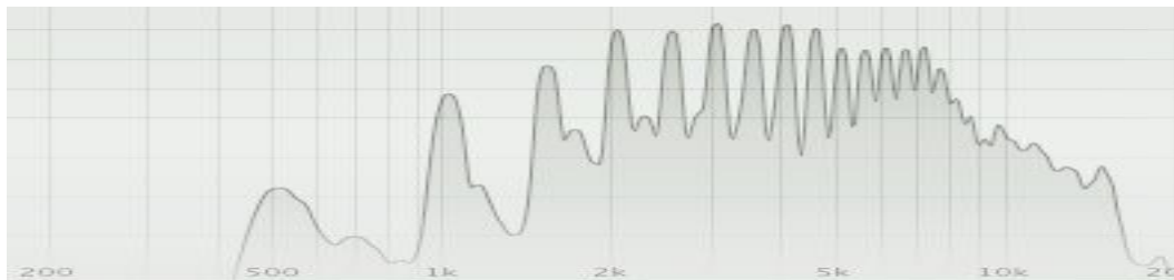
Figure 16. Frequency array of the suona (x-axis: frequency, y-axis: dB)
