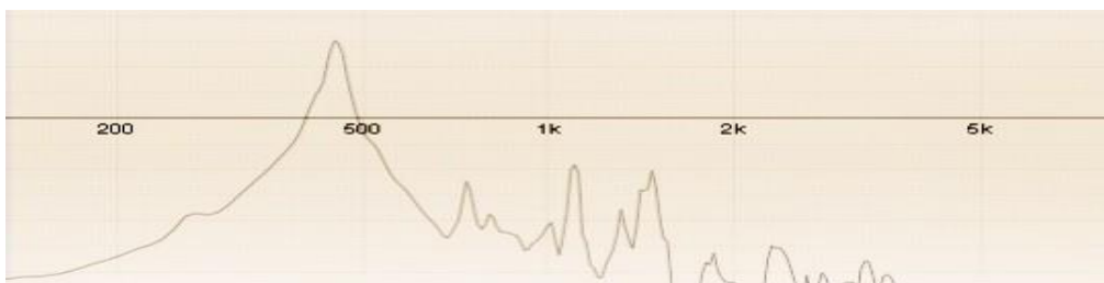
Figure 11. Frequency array of the tonggu (x-axis: frequency, y-axis: dB)
