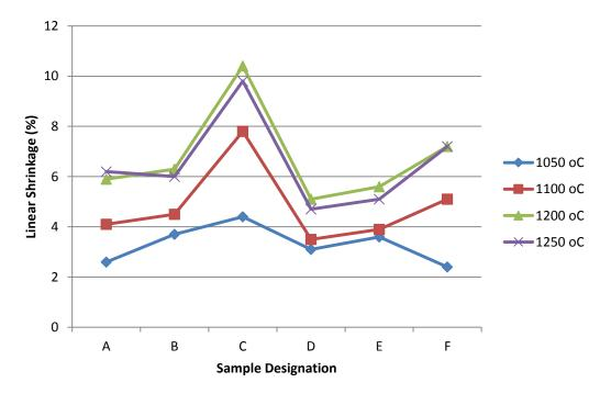
Figure 1. Linear shrinkage of samples sintered at different temperature
