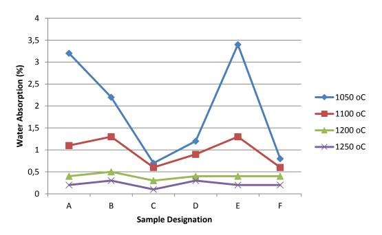
Figure 2. Water absorption of samples sintered at different temperature
