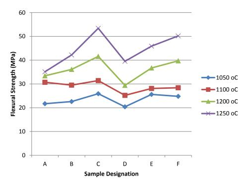
Figure 4. Flexural strength of samples sintered at different temperature
