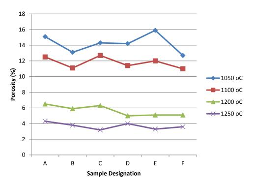
Figure 3. Porosity of samples sintered at different temperature
