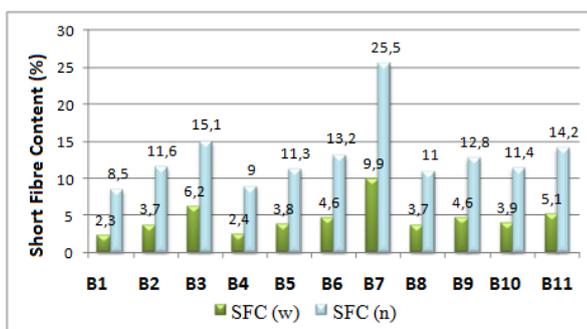
Figure 2. Short fibre content by weight and short fibre content by number values of the different blends
