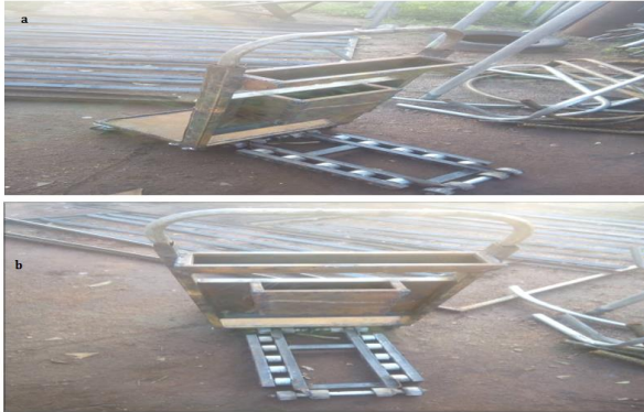
Figure 5. An assembled motorized staircase trolley.
