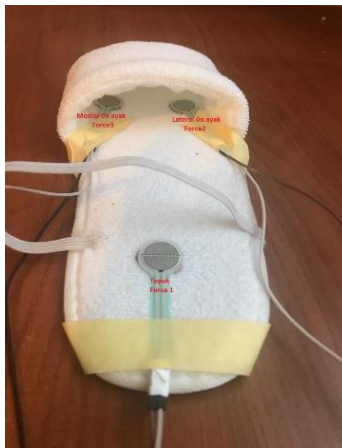
Figure 8. The placement of the sensors on the designed shoe
