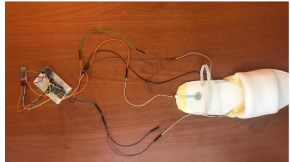
Figure 5. Developed smart shoe system
