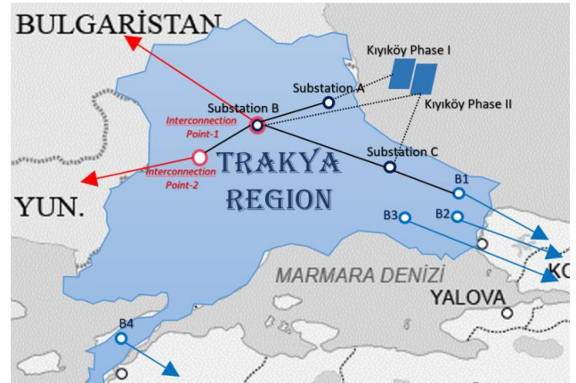
Fig. 1. Trakya Region and its connections with the rest of the grid. B1, B2, B3 and B4 are boundary busbars representing Trakya side ending points of the connection lines over the Bosphorus and Dardanelles. Substation A, B and C are denoting three connection busbars of OWPP (Strait connecting lines and grid interconnection lines are implemented with blue and red, respectively).
