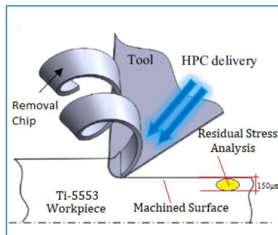
Figure 3. HPC processing and residual stress measured surface.
