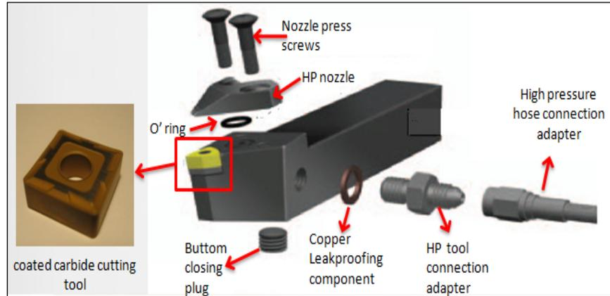
Figure 2. Cutting tool and HPC connection equipment
