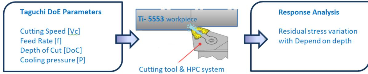
Figure 1. Schematic view of machining process.
