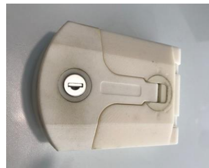
Fig. 5. 3D Printed Prototype Lock
