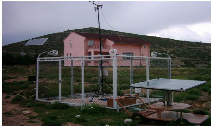
*Figure 5. PV and sun-tracking system for mobile meteorology station project*
