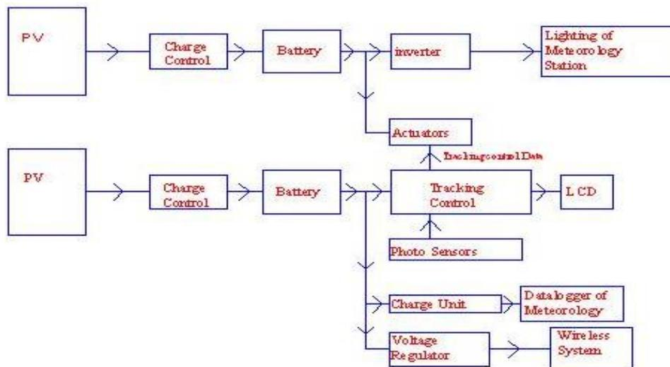
Figure 4. Block diagram for system
