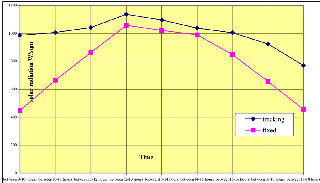
**Figure 6.** Average hourly solar radiation values, which are measured on tracking panels and fixed (25° south) panel surface 10.06.2005.
