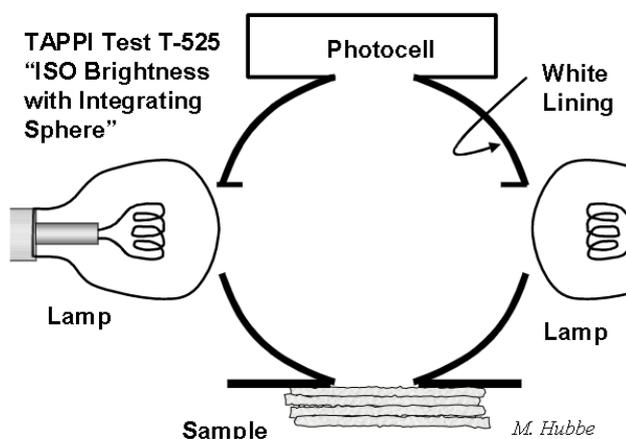
Figure 1. Basic configuration of paper brightness according to TAPPI Method T 452
