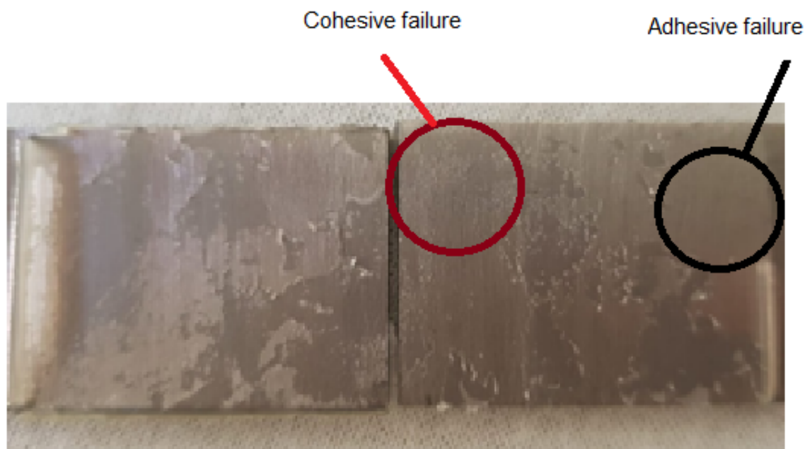
Figure 4. Mixed failure mechanism on debonding surface of specimen reinforced with 2wt.% NSPs.
