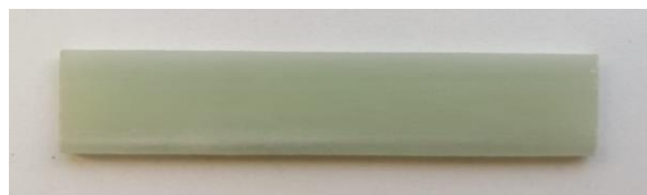
Figure 1 Three-point bending test sample
